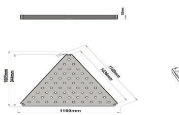
• PVC thickness is produced at a minimum of 2 mm at each point.
